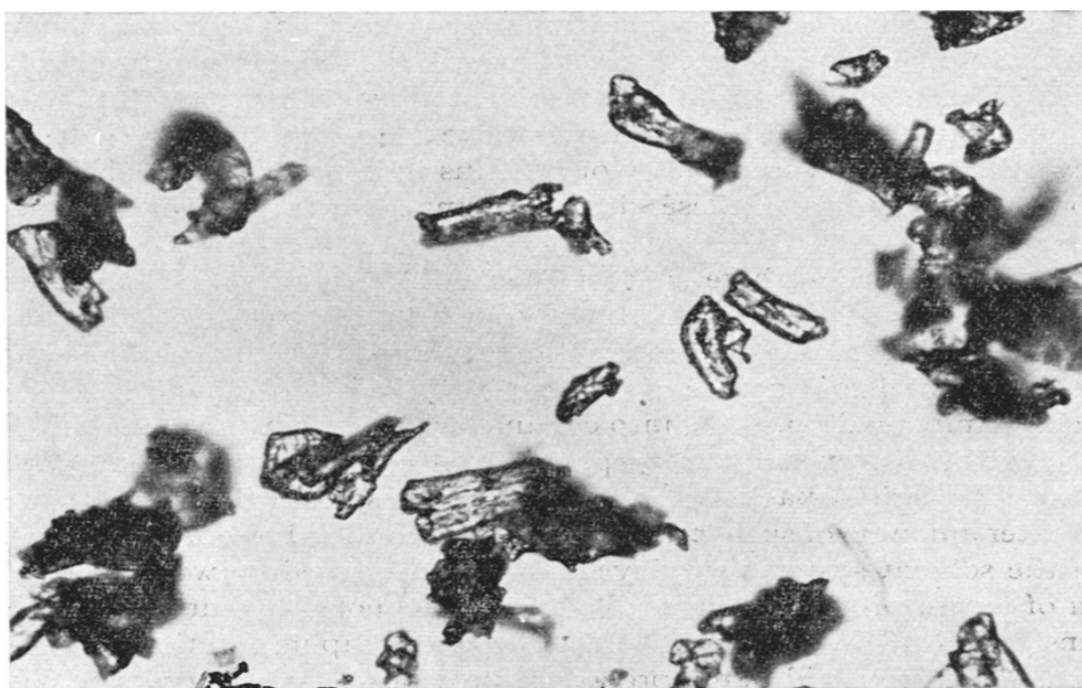
Fig. 6. Photomicrographs of "C" and "W" type exchangers. A. Exchanger C120, magnification \times 100 . B. Exchanger W, magnification \times 250 .
